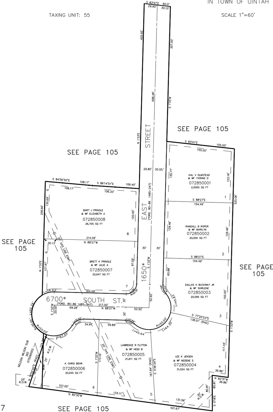
7' UTILITY & DRAINAGE EASEMENTS EACH SIDE OF PROPERTY LINE AS INDICATED BY DASHED LINES. UNLESS OTHERWISE SHOWN.
